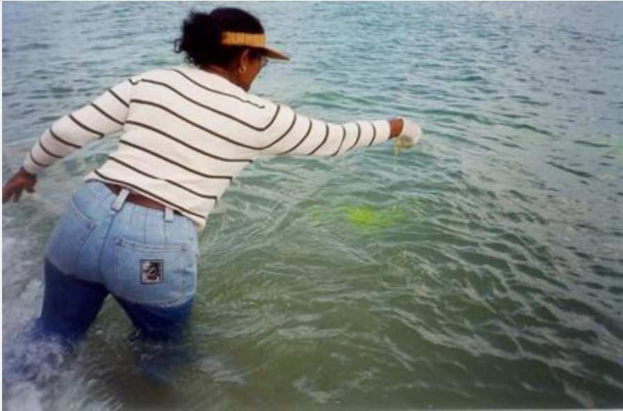
Putting fluorescent dye in the water to measure the currents
