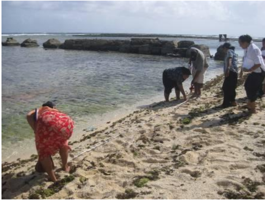
Measuring the longshore current
