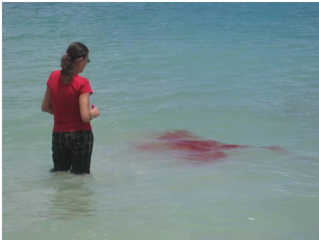
Tracking the longshore current using red dye
