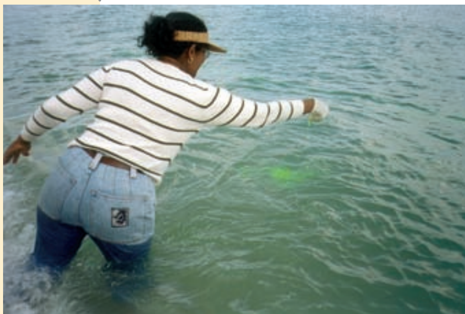
Measuring longshore currents with fluorescent dye.
