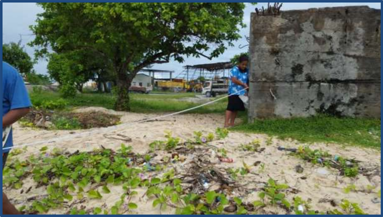
Measuring beach width from a reference point
