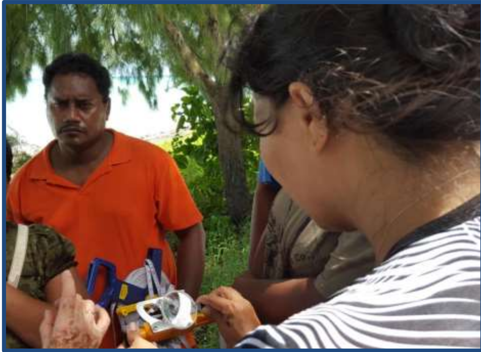
Reading the Abney level for beach profile measurements
