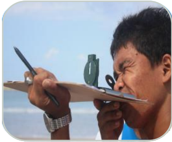
Measuring wave direction in Aceh, Indonesia. Photo courtesy of Jaringan KuALA
